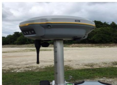
Gambar 2.16 *Receiver Pada Rover*
