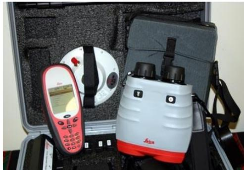
Gambar 2.8 Receiver Tipe Pemetaan Leica GS20.
