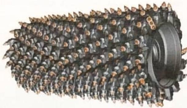
Gambar 2. 4 *Milling drum surface miner* (Google, 2023)
